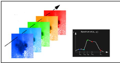
**Figure 1.** A spectral cube consists of a number of grayscale images showing intensity at every pixel as a function of wavelength. An optical spectrum is thus associated with each pixel.
