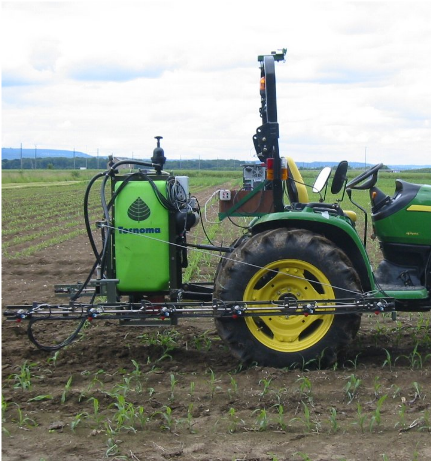
Figure 2. The real-time precision sprayer. Actuators are placed in front of each nozzle of the spraying boom and are activated according to the speed sensor and the image snapped by a camera mounted in front of the tractor.
