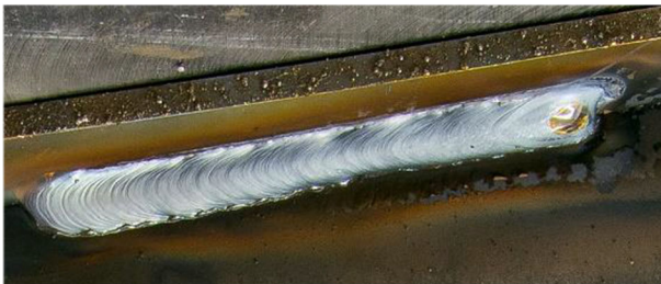
e) Colour image of a defect-free weld
