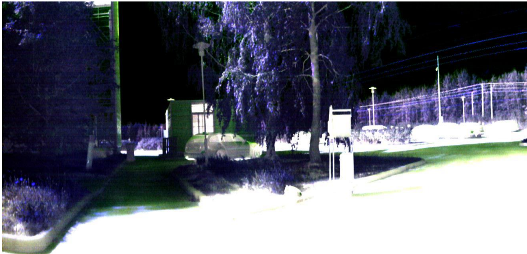
Figure 3: False RGB composite based on a FX50 data cube. The black body is clearly visible on the right hand side of the image (bright square).
