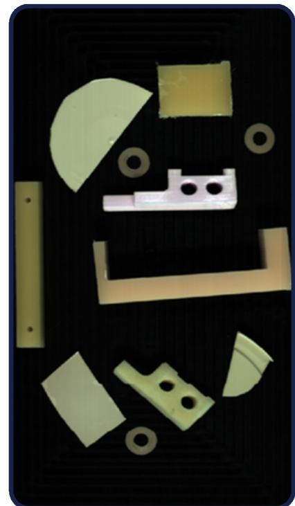
Once both datasets were collected, they were uploaded into SpecimINSIGHT. Two sets of selections were made for each plastic sample from the Training & Validation Dataset, as seen above; one larger selection used to train the model, and one smaller selection used for validation.
