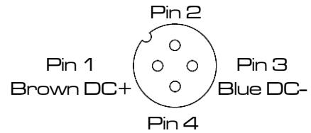
M12, 4 Pin Connector, Pin 1 +, Pin 3 -
