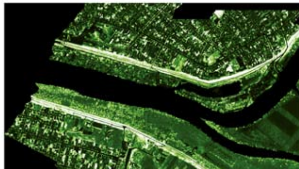
Normalized Difference Vegetation Index (NDVI) can be applied to estimation of water content in the terrain and assisting in the computation of risk maps
