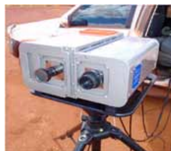
Dual VNIR and SWIR camera setup on a rotary scanner
