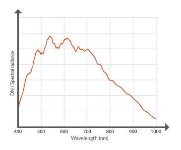
The Specim FX10+ is a high-speed line-scan hyperspectral camera optimized for applications requiring fast imaging. Its high resolution ensures accurate and detailed imaging at a rapid pace. Specim FX10+ operates in the visible and nearinfrared (VNIR) region from 400 to 1000 nm.
