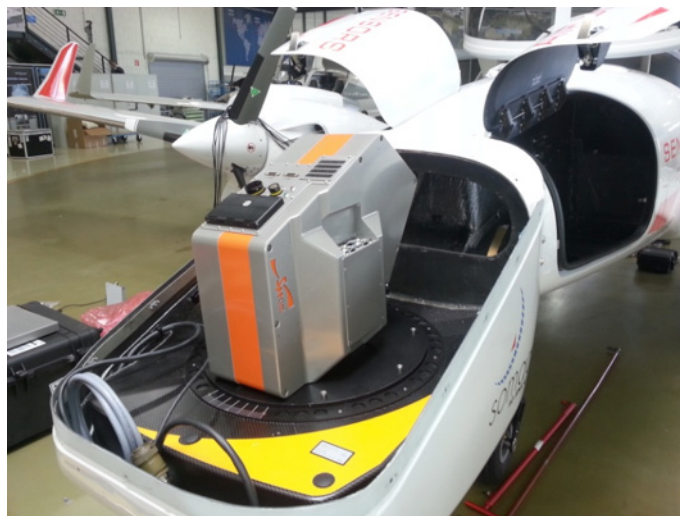
Nosepod of a DA42MPP with AisaFENIX mounted on gyrostabilized cameramount.
