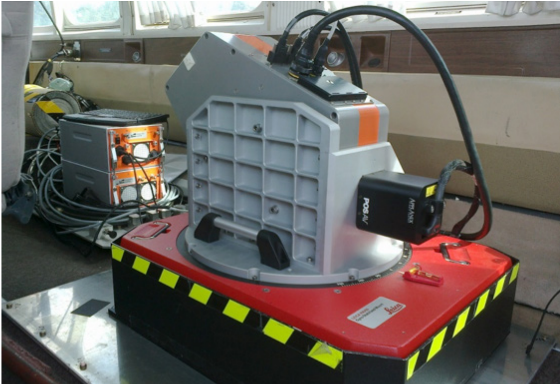
AisaFENIX mounted on a gyrostabilized mount.
