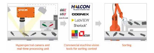
A line scan (push-broom) type spectral camera can be installed, together with proper line illumination and the real-time data processing solution, on existing and new sorting lines like any line-scan camera. The material identification result, pixel by pixel, is available through a standard interface (like Gen<I>Cam) to commercial machine vision systems. The results can then be used to control the air nozzles or picking robots.
